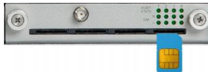
Fig: Inserting SIM in Cellular card.
